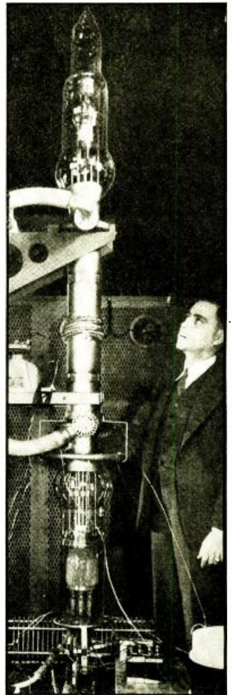
Fig. D. 1938's transmitter tube contribution to the electronic field, a 250,000-W. water-cooled giant.
